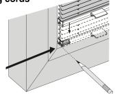
For blinds installed with Fixing Clips only, the lateral bracing cord is fastened with Horizontal Mounts.
