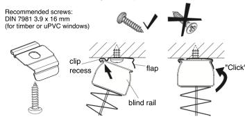
Insert the edge of the blind rail diagonally into the clip recess, then straighten upwards until the rail 'clicks' into place.
