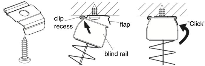
Insert the edge of the blind rail diagonally into the clip recess, then straighten upwards until the rail 'clicks' into place.
