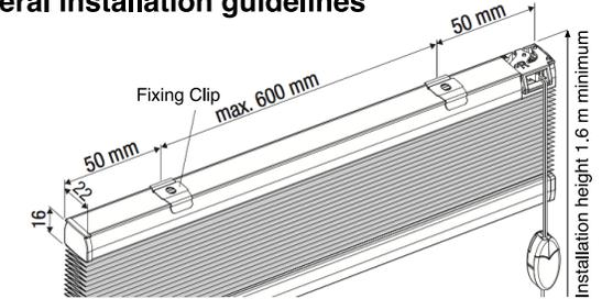
Install Fixing Clips 50 mm from each end of the rail, and with a maximum spacing of 600 mm between clips.
