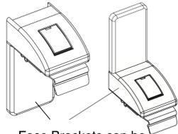
Face Brackets can be installed with legs turned upwards or downwards.
